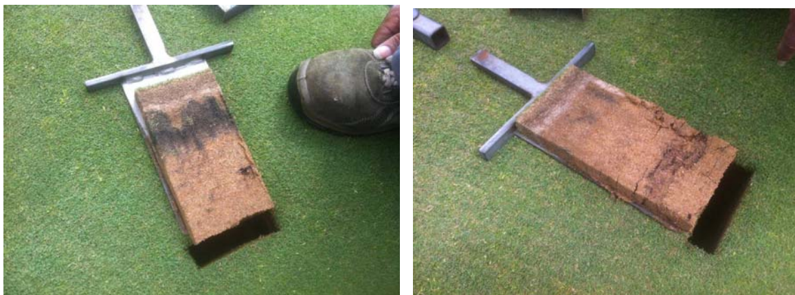
Pictures 2 & 3. Different composition in root profile seen in different areas of greens
